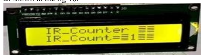
Fig 16: LCD is displaying the no. of people entering the
