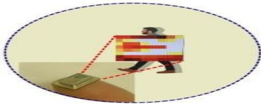
Fig 11. Infrared sensor for tracking human passage movement
